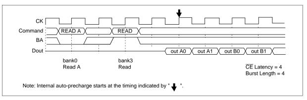
Read with Auto Precharge to Read Command Interval (Different bank)
